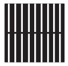
Half-cell with MBB design decreases internal resistance while boosts power output; narrowed inter-cell gap through flexible welding technology contributes to the module's compact dimension.
